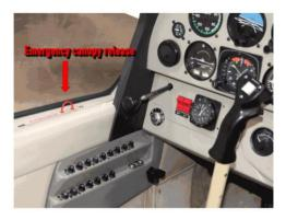
**Emergency release** - There are two emergency release levers at the forward ends of the canopy to allow the canopy to be jettisoned altogether in an emergency. They must never be moved except in an emergency and even then, not in flight!
